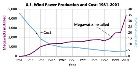
**Figure 6** ► The cost of wind power has been steadily falling as wind turbines have become more efficient.
